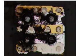
Damaged Electrodes of the LED chip due to an Inrush Current.
