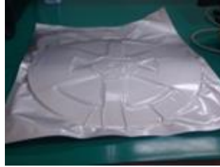
Squashed Reel as a Result of Excessive Vacuum Sealing
