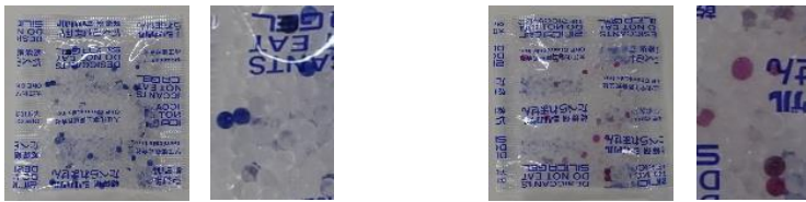
B. After being left for 168 hours at 30^\circ\text{C} and 70%RH
