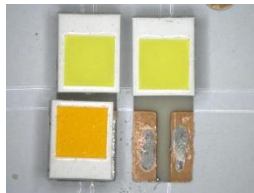
b) Solder Printing Failure Resulting in Open Circuit/LED Removal from the PCB
