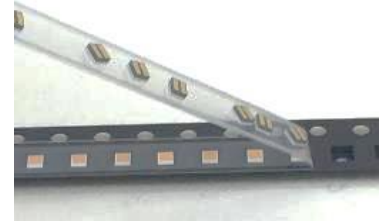
Figure 18. LED Sticking due to Static Charge
