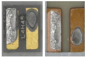
a) Solder Printing Failure Resulting in a Reduction in the Luminous Flux of the LED
