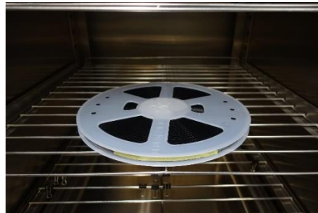
Figure 5. Example for Baking the LEDs
